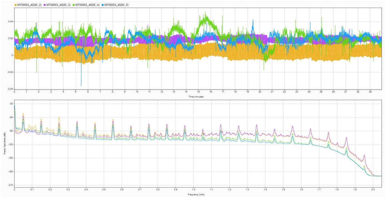
Figure 3: Time series (top panel) and power spectra (bottom panel) related to the Electric ( E_x and E_y ) and Magnetic ( H_x and H_y ) field components sampled at 4096 Hz. E_x is plotted in ochre, E_y in purple, H_x in green and H_y in cyan. The components were measured in the (magnetic) N-S and E-W directions. The signal was analyzed in Matlab® Signal Processing Toolbox.
