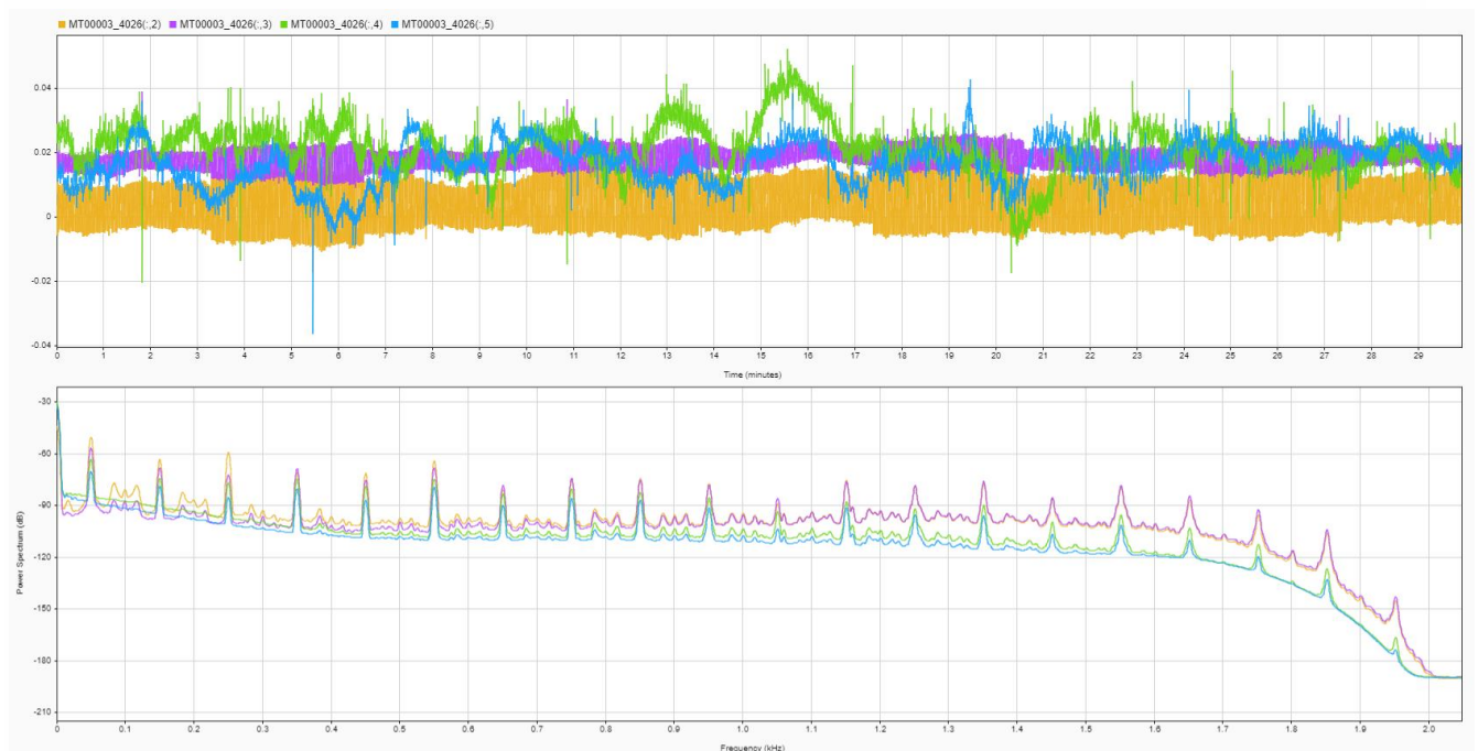
Figure 3: Time series (top panel) and power spectra (bottom panel) related to the Electric (Ex and Ey) and Magnetic (Hx and Hy) field components sampled at 4096 Hz. Ex is plotted in ochre, Ey in purple, Hx in green and Hy in cyan. The components were measured in the (magnetic) N-S and E-W directions. The signal was analyzed in Matlab® Signal Processing Toolbox.
