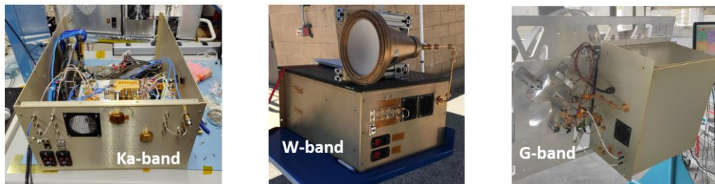
90 Figure 1: Pictures of the CloudCube rack-mounted prototype modules operated during the EPCAPE deployment. From left to right: the Ka-band, W-band and G-band CloudCube radar channels.
