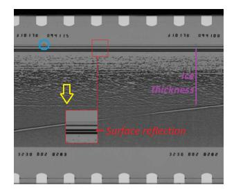
**Figure 7.** Image file 13\_0014525\_0014550\_lowqual.jpg from flight line 2, 1978, 60 MHz. The yellow arrow indicates the bed reflection. The insert outlined in red is an enlargement of the surface reflections. The blue circle indicates the exact location of the coordinates tied to CBD 283.
