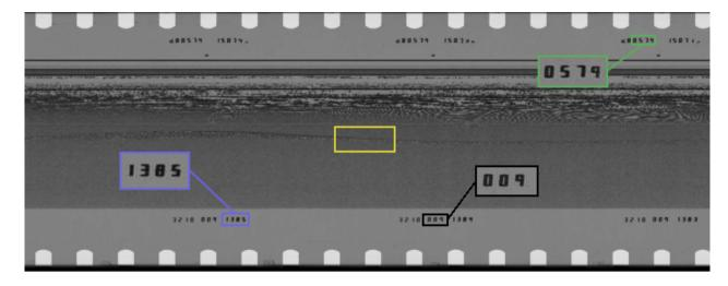
**Figure 4.** Example of a radargram. The green box indicates the date of acquisition (month and year) in this case May 1979, the black box shows the flight line number (flight line 9), and the blue box indicates the location of the CBD. The yellow box shows the location of the bed reflection. This radargram spans CBDs 1383 to 1385 corresponding to approximately 5.6 km.
