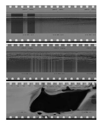
**Figure 9.** Example of radargrams acquired in 1979 from flight lines 9, 10, and 8, respectively. The radargrams exemplify different known data quality issues, such as, variations in brightness along a flight line, the occurrence of stripes, and errors introduced during the development of the films. The radargrams all span approximately 5.6 km.
