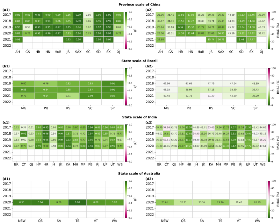
Figure 10: Comparison between identified and statistical areas of winter-triticeae crops at state (province) scale from 2017 to 2022. (a1-d1) represent the correlation coefficient at state (province) scale in China, Brazil, India, and Australia, respectively; (a2-d2) represent the RMAE at state (province) scale in China, Brazil, India, and Australia, respectively.
