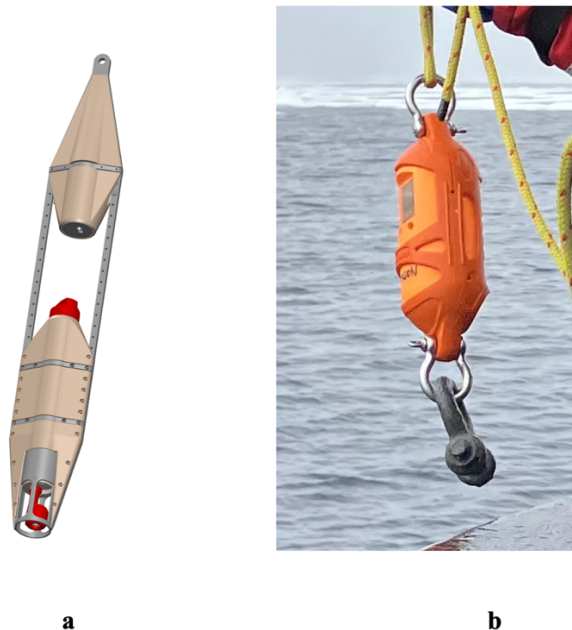
Figure 12. (a) uCTD and (b) cCTD instruments. The uCTD has a total length of 1.08 m and the cCTD a total length of 0.20 m.
