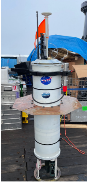
Figure 33. The UIF on the deck of the Woldstad before deployment. The float is about 2 m tall from the deck to the top of the antennas. Note CTDs at top and bottom of the float, upward-looking camera mounted near the top of the float body on the left, and an ice-profiling sonar attached to the right-hand side. Photo credit Jim Thomson.
