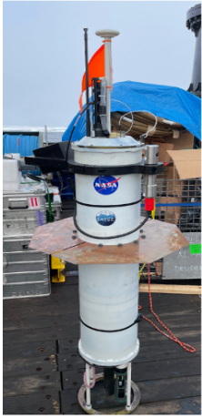
545 Figure 332. The UIF on the deck of the Woldstad before deployment. The float is about 2 m tall from the deck to the top of the antennas. Note CTDs at top and bottom of the float, upward-looking camera mounted near the top of the float body on the left, and an ice-profiling sonar attached to the right-hand side. Photo credit Jim Thomson.
