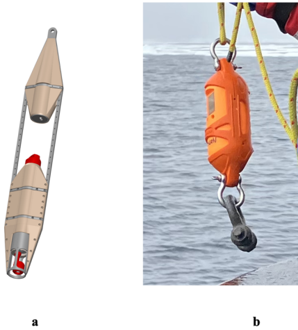
Figure 1212. (a) uCTD and (b) cCTD instruments. The uCTD has a total length of 1.08 m and the cCTD a total length of 0.20 m.
