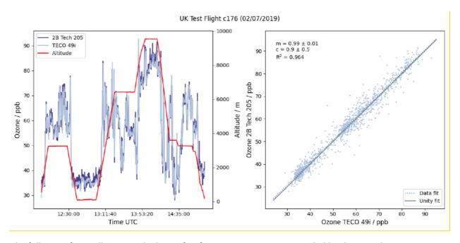
The following figure illustrates the linear fit of ozone mixing ratios recorded by the two photometers, averaged to 4 seconds (the Model 49i measurement rate) and weighted with uncertainties (3% or 3 ppb), for 28 missions flown by FAAM between 02/07/2019 and 14/02/2020.
