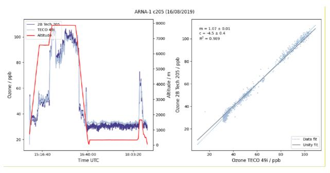
We have investigated this bias in our laboratories in 2020 and found it is related to the behaviour of the Dewlines/Nafion<sup>TM</sup> water exchange membrane technology employed in the 2B photometer with changing humidity. This issue has also been identified by Eric Hintsa at the NOAA Global Monitoring Laboratory (https://doi.org/10.5194/amt-14-6795-2021), who fly the UCATS payload also utilising 2B
