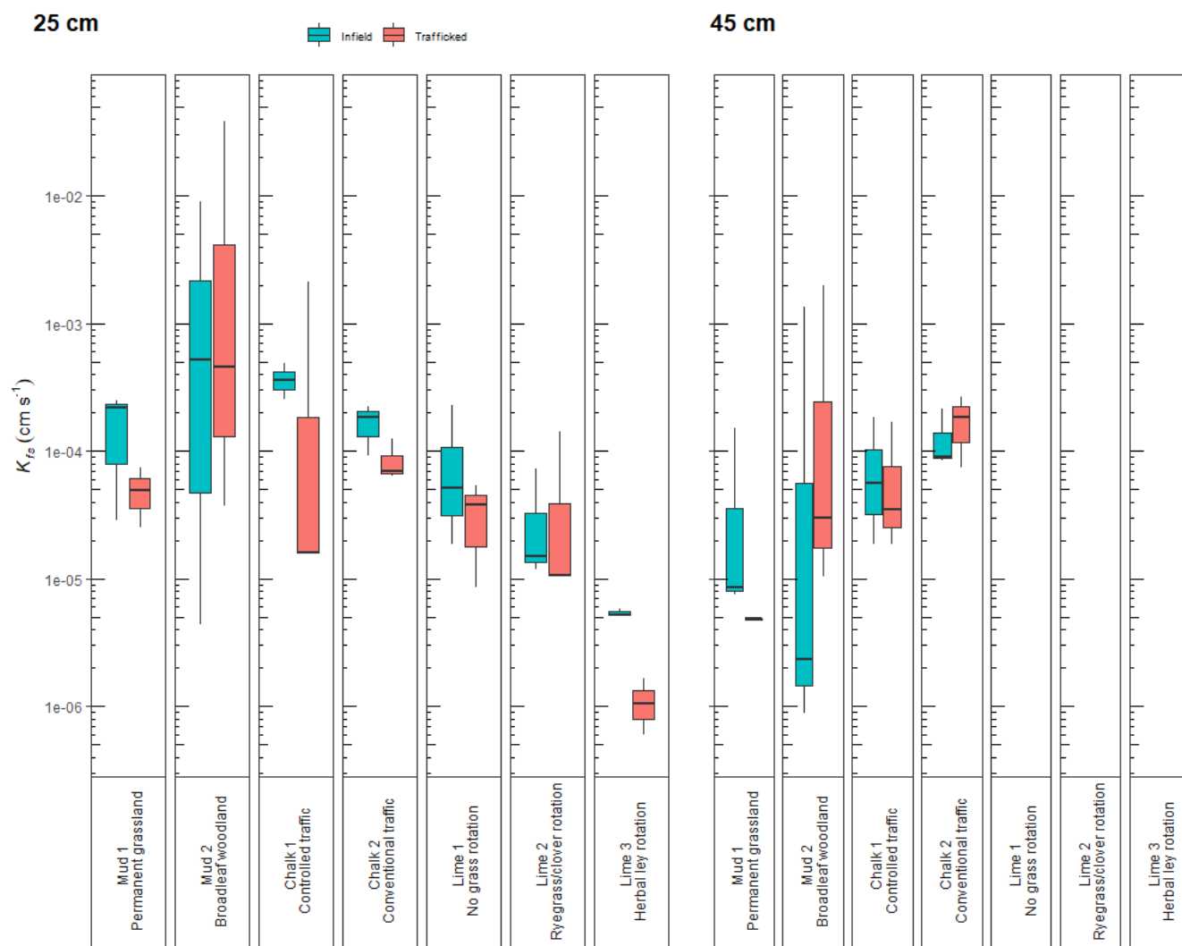
340 Figure 4: Box plots of saturated hydraulic conductivity ( K_s ) ( \text{cm s}^{-1} ) measurements taken at infield and trafficked locations at 25 cm 345 depth, and also 45 cm depth where possible. Bold lines indicate median values. Note the log scale.
