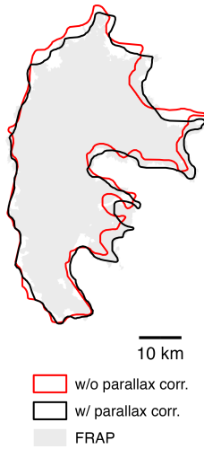
Figure B3. Effect of the parallax terrain correction on the final perimeter, using the Creek Fire as an example. The final perimeter of the Creek Fire with the parallax correction (red polygon) and without parallax correction for GOFER-Combined is shown alongside the FRAP perimeter (black polygon). For the uncorrected perimeter, we use a confidence threshold of 0.91, which yields the highest mean IoU among the 10 largest CA fires in 2020 when the parallax adjustment factor is zero (Fig. 4a).
