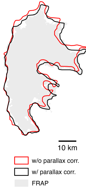
Figure B3: Effect of the parallax terrain correction on the final perimeter, using the Creek Fire as an example. The final perimeter of the Creek Fire with the parallax correction (red polygon) and without parallax correction for GOFER-Combined is shown alongside the FRAP perimeter (black polygon). For the uncorrected perimeter, we use a confidence threshold of 0.91, which yields the highest mean IoU among the 10 largest CA fires in 2020 when the parallax adjustment factor is 0 (Figure 4a).
