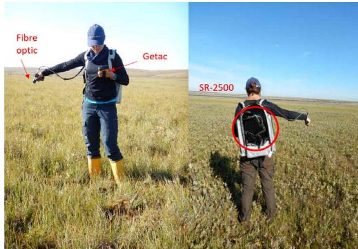
Figure S2: Spectral Evolution SR-2500 field-spectrometer measurement set-up in the Lena Delta, August 2018 (photos: M. Fuchs).
