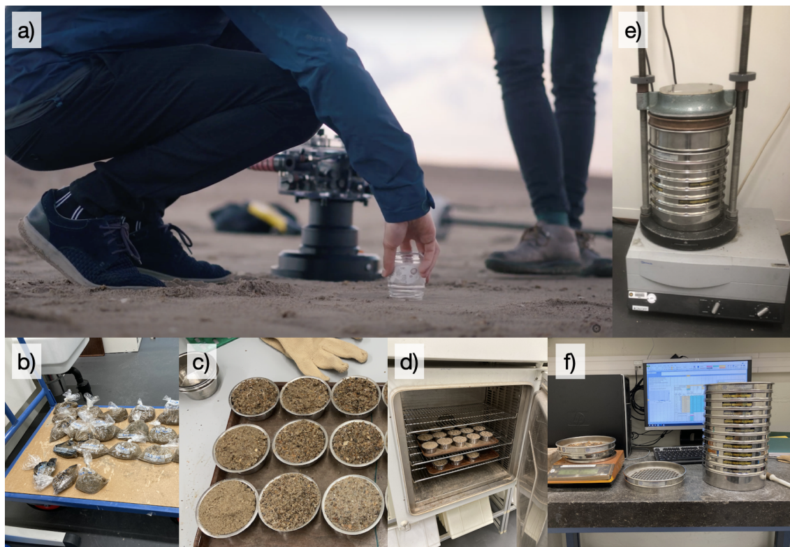
Figure 5. Sediment-analysis procedure: (a) sample with a small glass jar, (b) collect material in plastic bag, (c) collect sub-sample inside aluminium cup, (d) dry sub-samples in oven, (e) shake sub-sample in sieve tower and (f) weigh each sieve with retained material.
