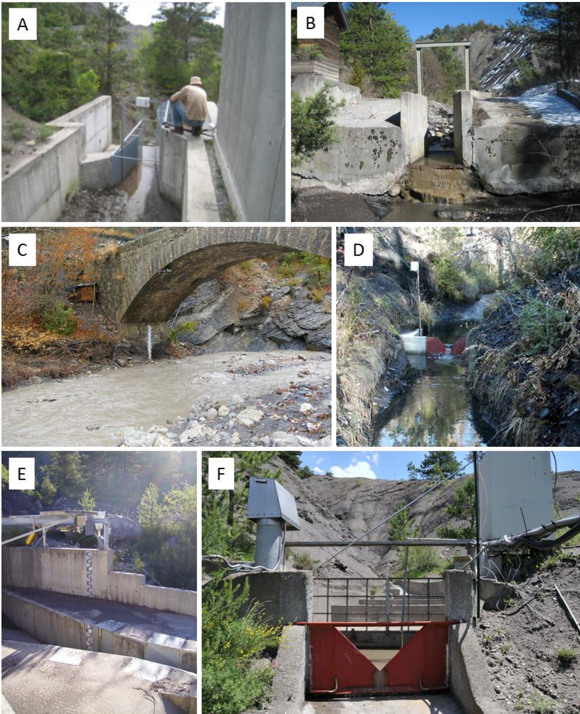
Figure 7: Photos of all the stations: A) Moulin Parshall flume. B) Francon Parshall flume looking upstream. C) Bouinenc natural gauging section. D) Brusquet low-discharge weir. E) Laval Parshall flume. F) Roubine weir looking upstream (photo F from J. Latron)
