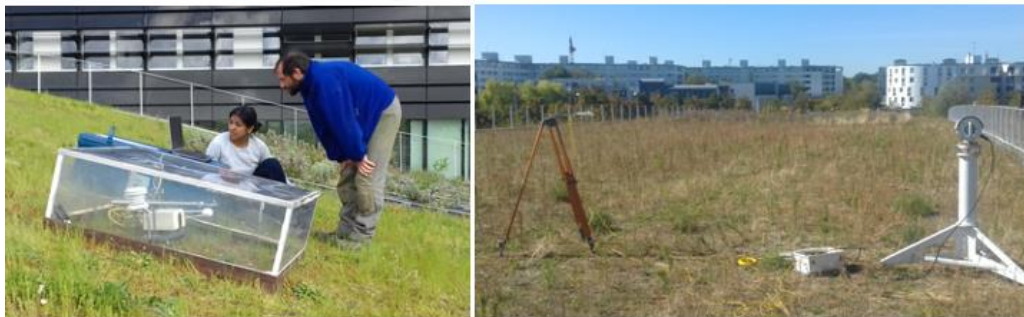
Figure 1. The Blue Green Wave experimental site: implementation of the different sensors (top), the evapotranspiration chamber (bottom-left), and the surface energy balance instruments (bottom-right)
