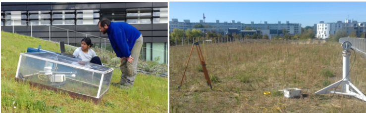
135 Figure 1. The Blue Green Wave experimental site: implementation of the different sensors (top), the evapotranspiration chamber (bottom-left), and the surface energy balance instruments (bottom-right)
