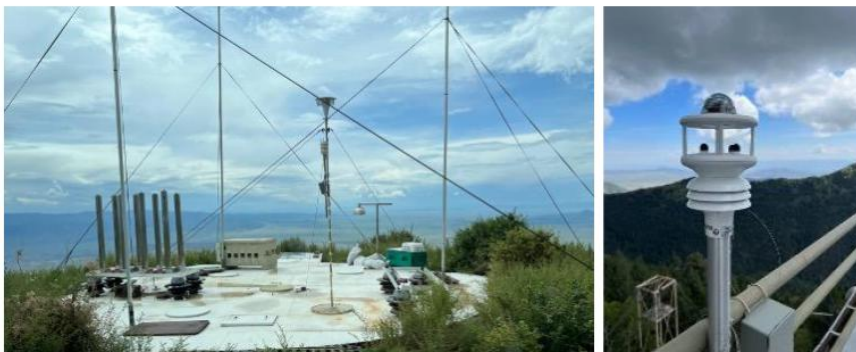
Figure 4. Photographs of aerosol detectors and automatic weather station locations on the Magdalena mountains during the DCMEX campaign. (Left) Kiva-2 Laboratory rooftop, South Baldy Peak, includes a centrally mounted University of Manchester Aerosol Inlet with Sigma-2 inlet, and Vaisala WXT536 Meteorology Station. (Right) Gill MaxiMet GMX600 Meteorology Station (University of Manchester) mounted on the Langmuir laboratory rooftop railing.
