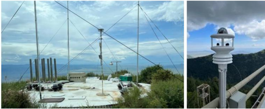
Figure 4. Photographs of aerosol detectors and automatic weather station locations on the Magdalena mountains during the DCMEX campaign. (Left) Kiva-2 Laboratory rooftop, South Baldy Peak, includes a centrally mounted University of Manchester Aerosol Inlet with Sigma-2 inlet, and Vaisalla WTX536 Meteorology Station. (Right) Gill MaxiMet GMX600 Meteorology Station (University of Manchester) mounted on the Langmuir laboratory rooftop railing.
