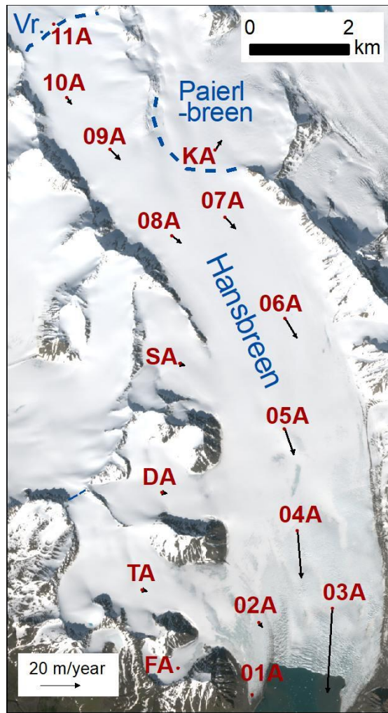
Figure 5. Mean annual horizontal velocities for the hydrological year 2006-2007, as an example of the spatial pattern of Hansbreen velocity. The stakes 11 and K flow into other ice masses. Vr. stands for Vrangpeisbreen. Background: Sentinel2 (2018-07-06).
