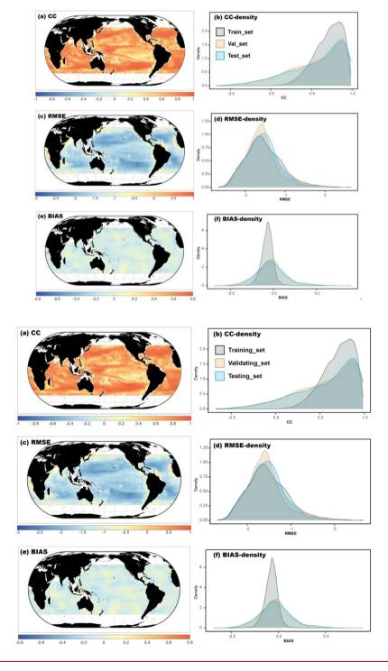
Figure 7 Evaluation results of OCNET based on the NOAA MSL12 dataset. a), c), and e) represent the global distribution maps of CC, RMSE, and bias from February 9, 2018, to December 31, 2021, respectively. b), d), and f) display the density distributions of
