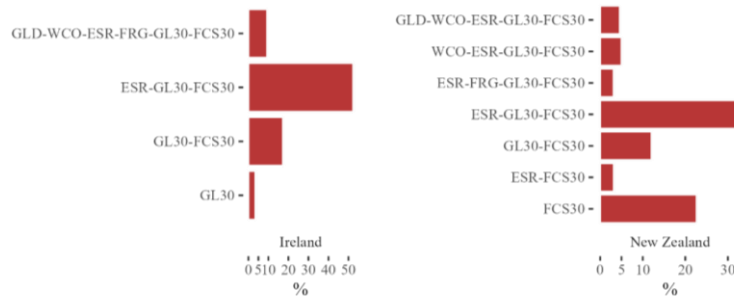
Figure 8. Percent contribution of products combinations to the detailed agreement, in Ireland and New Zealand. (Detailed agreement limited to land cover combinations with at least 3% contribution. ESR=ESRI; FCS30=GLC_FCS30-2020; FRG=FROM_GLC Plus; GLD=GLAD; GL30=Globeland30; WCO=WorldCover).
