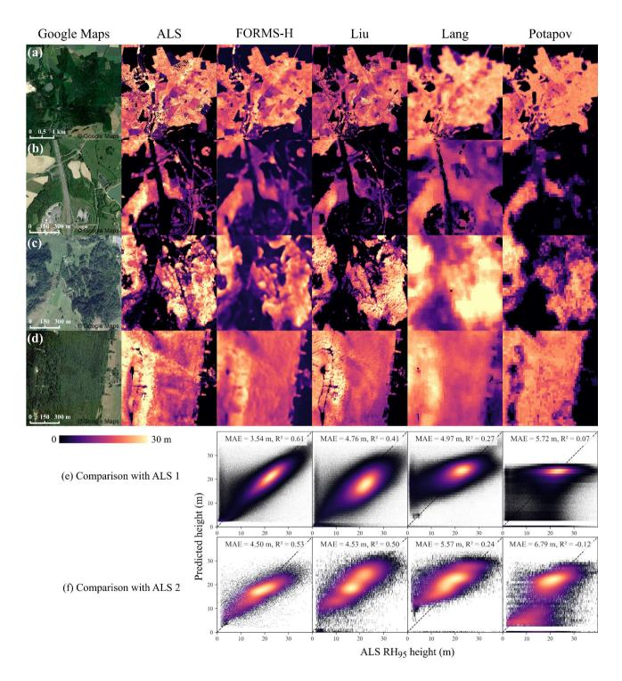
Figure 6: Visual (a,b,c,d) and quantitative (e,f) comparison of ALS RH<sub>95</sub> height data resampled at 10 m resolution to FORMS-H (10 m resolution) and to three other products at 3 m (Liu et al., 2023), 10 m (Lang et al., 2022) and 30 m resolution (Potapov et al.,
