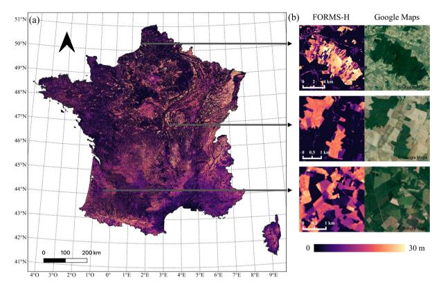
225 Figure 4: (a) FORMS-H: Tree height map of France at 10 m resolution for the year 2020. (b) Examples at three different locations of height prediction (left) with the corresponding Google map images from 2020, 2018, and 2019 (right). Brighter colors indicate higher heights.
