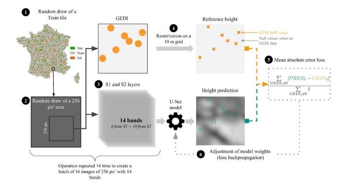
120 Figure 1: U-Net training process. (1) Random draw of a train tile (2) Random draw of a 2560x2560 m subset (3) Input of the corresponding S1 and S2 layers to the model. (4) Rasterization of the corresponding GEDI data on a 10 m grid. (5) Calculation of the MAE loss (6) Loss backpropagation: Model weights are modified according to the value of the loss gradient with respect to them.
