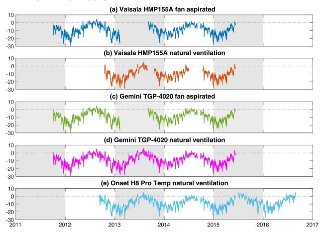
Figure 5. Daily mean air temperature series measured by different sensors installed at the Automatic Weather Station on Mt. Ortles.
