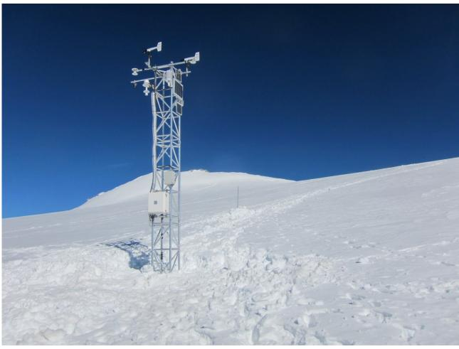
Figure F1. The automatic weather station (AWS) installed on Mt. Ortles, whose summit is visible in the background. The stake behind the weather station indicates the site of the Geoprecision thermistor string. Photo taken on 7 September 2012, after the lengthening of the support tower.
