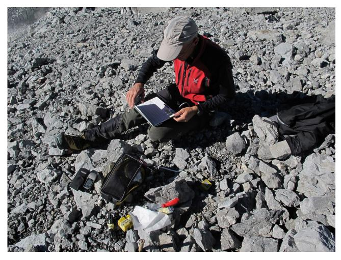
Figure H2. Data download and logger maintenance at the ORTL\_10 soil surface temperature site on 28 August 2012.
