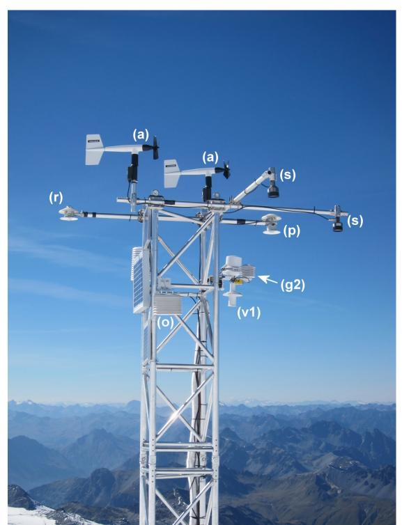
Figure F4. Detail of the AWS seen from the east: a) R. M. Young 05103 anemometers, p) Delta Ohm LP PIRG 01 pyrgeometers, r) Delta Ohm LP Pyra 05 radiometers, s) Campbell Scientific SR50A snow depth sensors,
