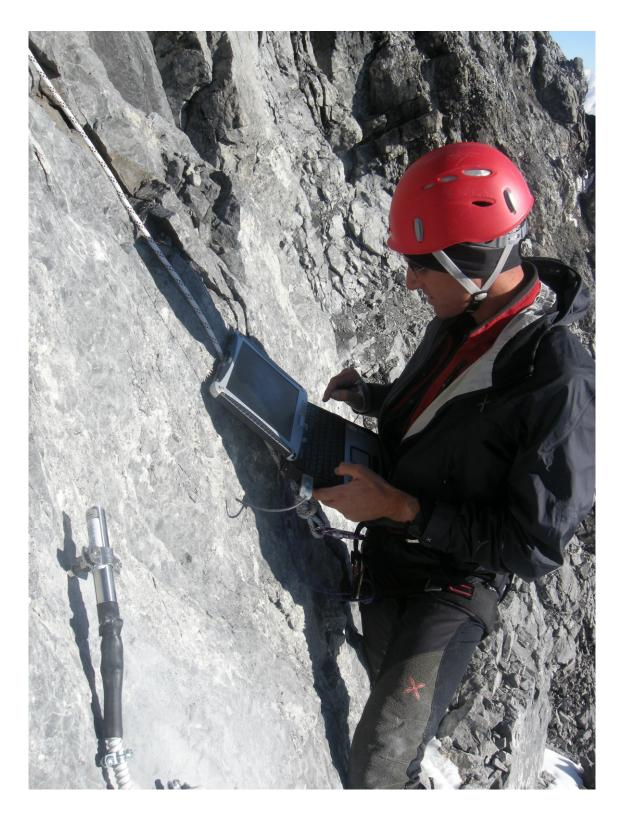
Figure I2. Launching of the CIMA ALTO data logger. A wireless USB dongle secures the wireless connection to the laptop used for launching the logger and for downloading the temperature data. Photo taken on 30 August 2011.
