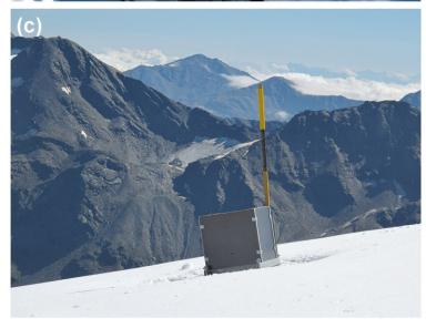
Figure G4. a) Borehole drilling at the Hintergrat Glacier using a steam ice drill. b) The box containing the winding system, the thermistor string data logger and the batteries. c) Final arrangement of the box housing the winding systems and the data logger. Photos taken on 17 November 2011 and 27 August 2015.
