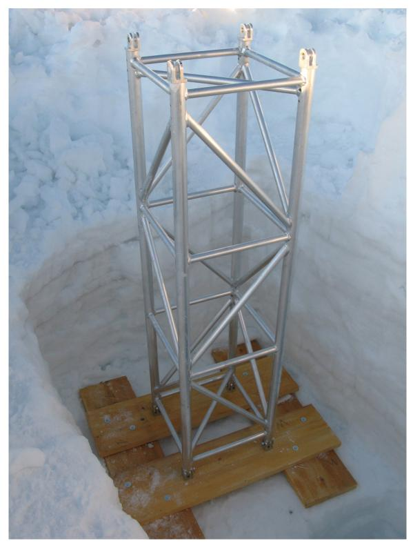
Figure F2. The wooden boards placed at the bottom of the support aluminum tower, at 2 m depth in the firn,
