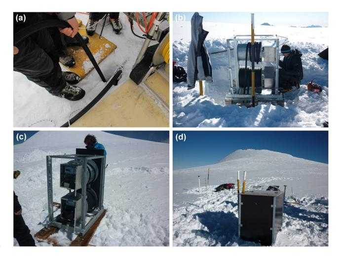
Figure G3. a) Lowering of a thermistor string into the borehole n. 3 at the drilling site. b) The winding systems of the two thermistor strings installed at the drilling site. c) The two metal boxes containing the thermistor string data loggers and the batteries. d) Final arrangement of the box housing the winding systems and the data loggers. The summit of Mt. Ortles is visible in the background. Photos taken on 17 November 2011.
