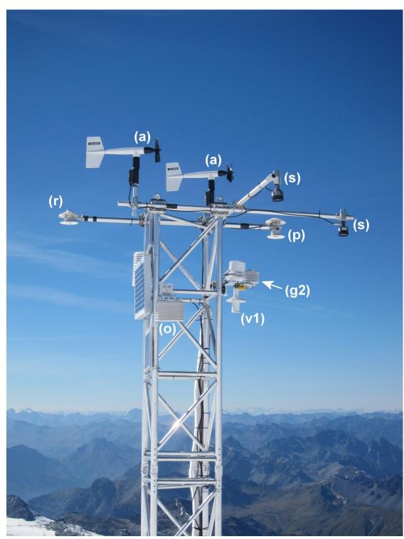
Figure F4. Detail of the AWS seen from the east: a) R. M. Young 05103 anemometers, p) Delta Ohm LP PIRG
