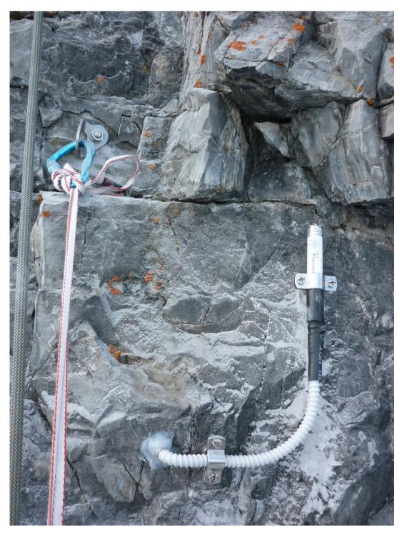
Figure I1. The rock wall temperature datalogger (Geoprecision thermistor string) installed close to the Payer
