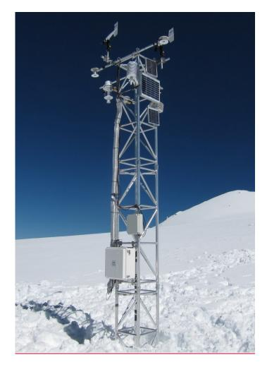
Figure 3. The automatic weather station installed in the upper accumulation area of Alto dell'Ortles Glacier.
