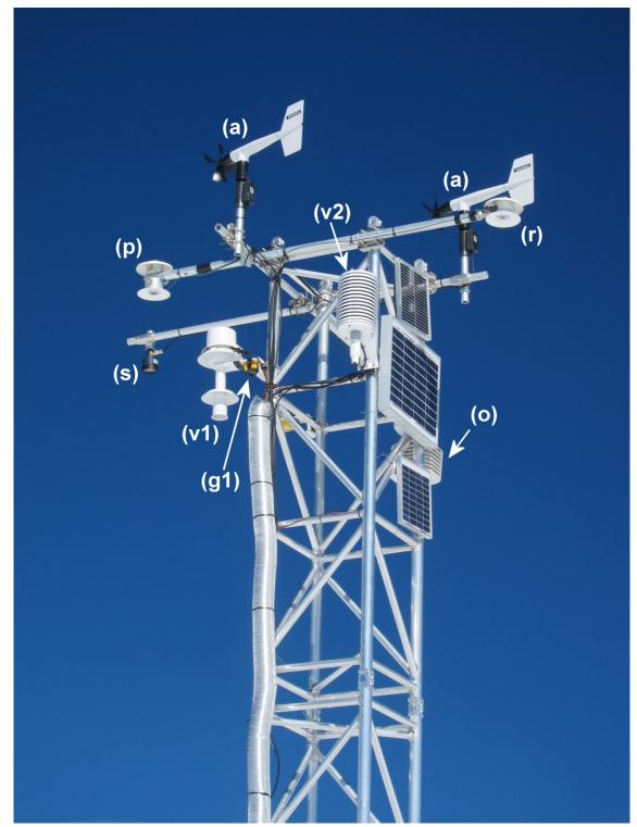
Figure F3. Detail of the AWS seen from the west: a) R. M. Young 05103 anemometers, p) Delta Ohm LP
