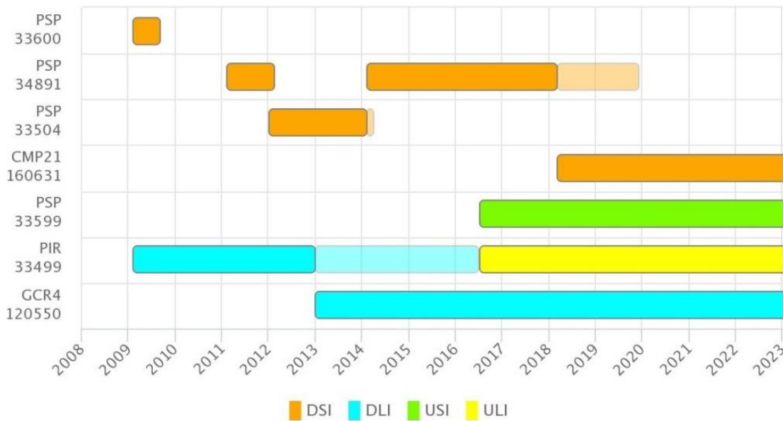
Figure 12: Radiometers installed at THAAO in the whole period 2009-2022. Shaded areas represent periods when a radiometer was tested by comparison with one having a fresh calibration.
