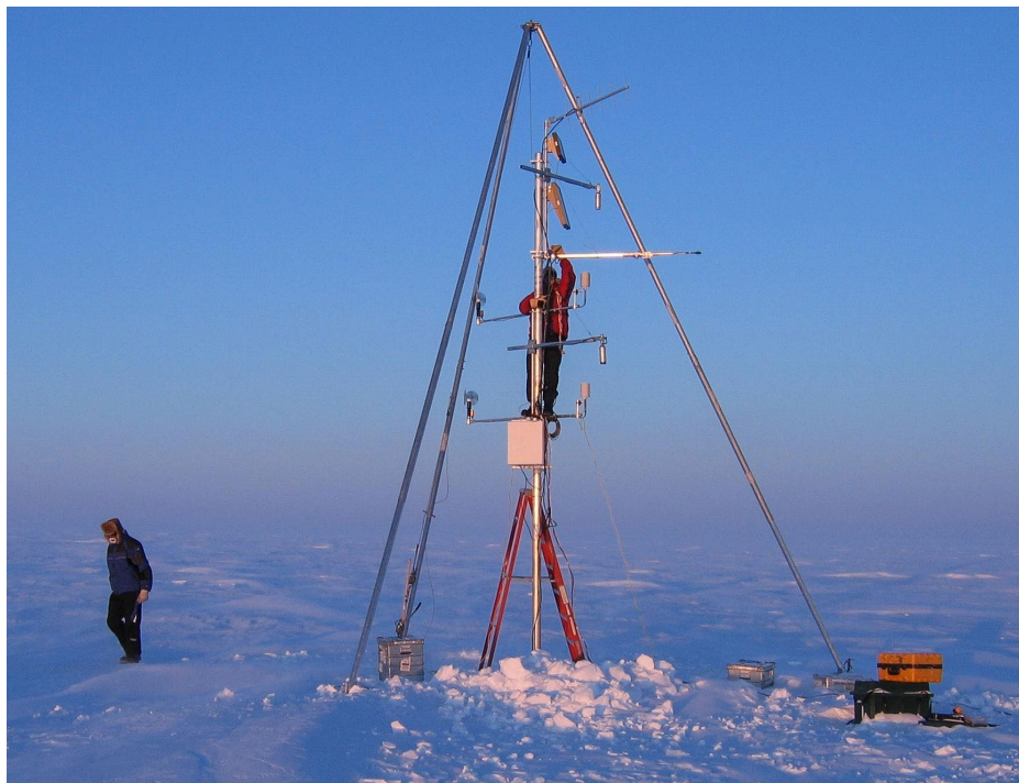
240 Figure 2. Raising the Crawford Point 1 mast, 3 May 2005. K. Steffen (left), R. Huff (right). Photo J. Box.
