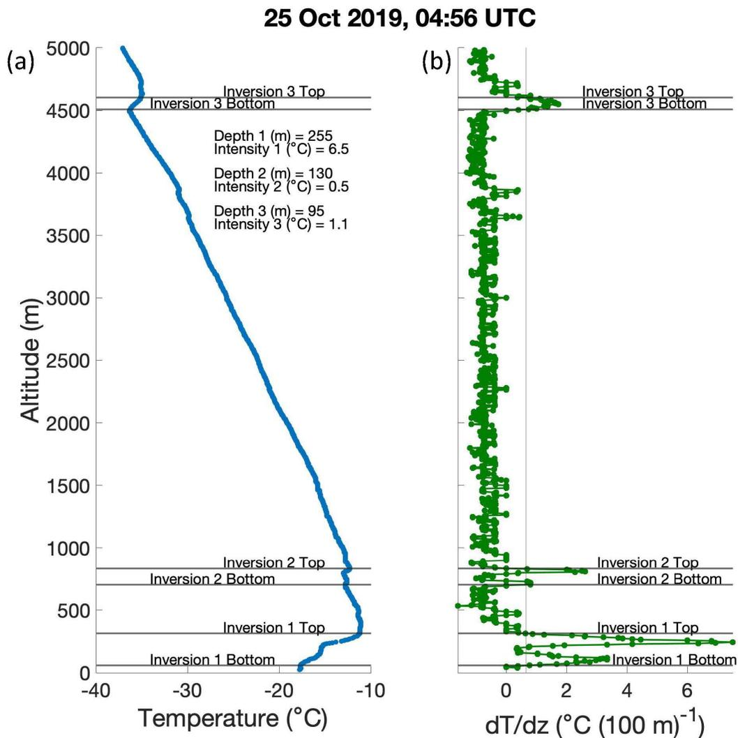
**Figure 2.** Example of temperature inversion identification using radiosonde profile at 04:56 UTC on 25 October 2019. Horizontal black lines on the (a) temperature profile and (b)  $dT/dz$  profile indicate the bottom and top of each TI. Vertical black line on the  $dT/dz$  profile indicates the threshold of  $0.65 \text{ }^\circ\text{C} (100 \text{ m})^{-1}$ . The depth and intensity of each inversion are written on the temperature profile plot.
