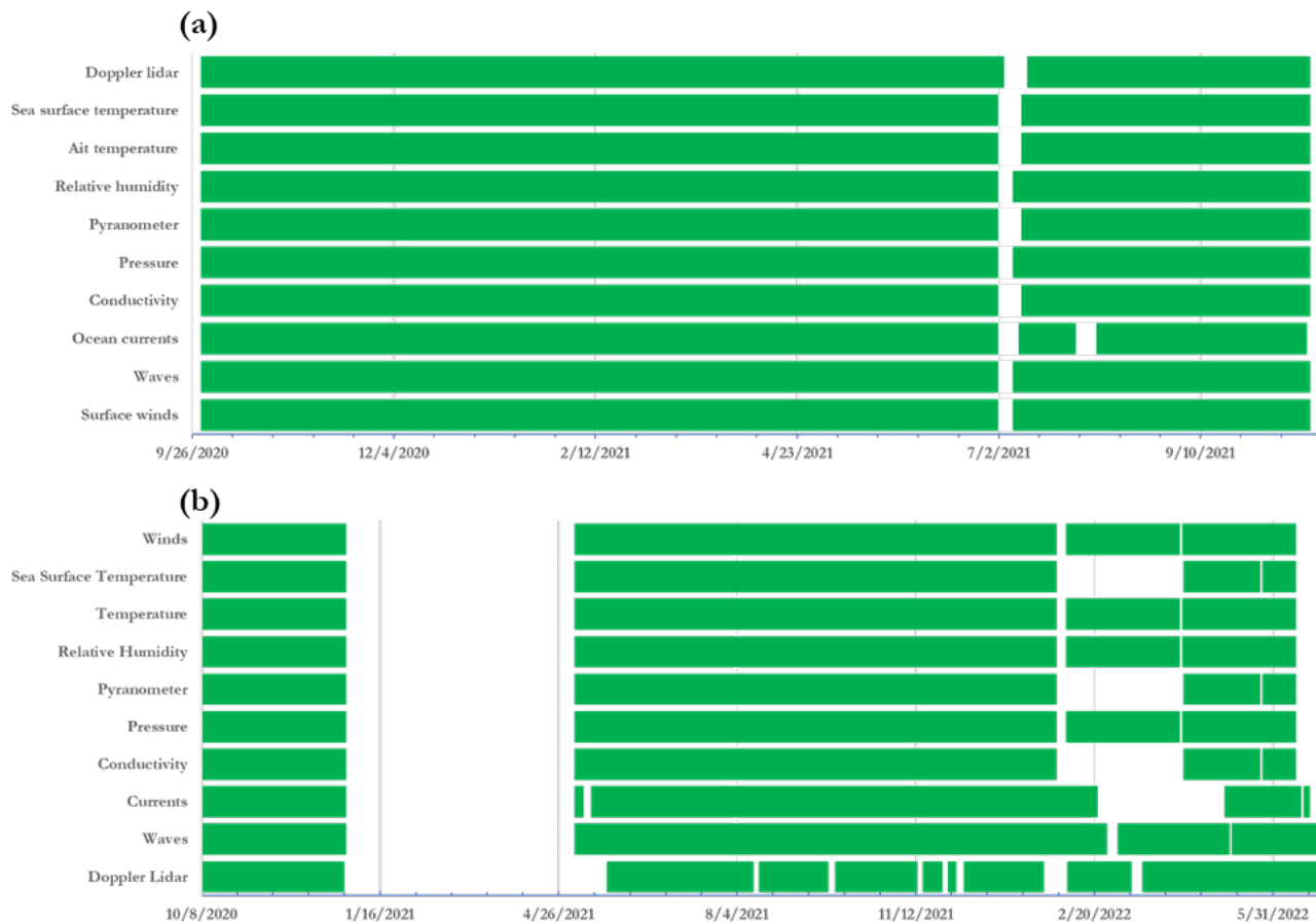
160 Figure 3: (a) Instrument uptime at Morro Bay for various instrument sensors and (b) instrument uptime at Humboldt for various sensors.
