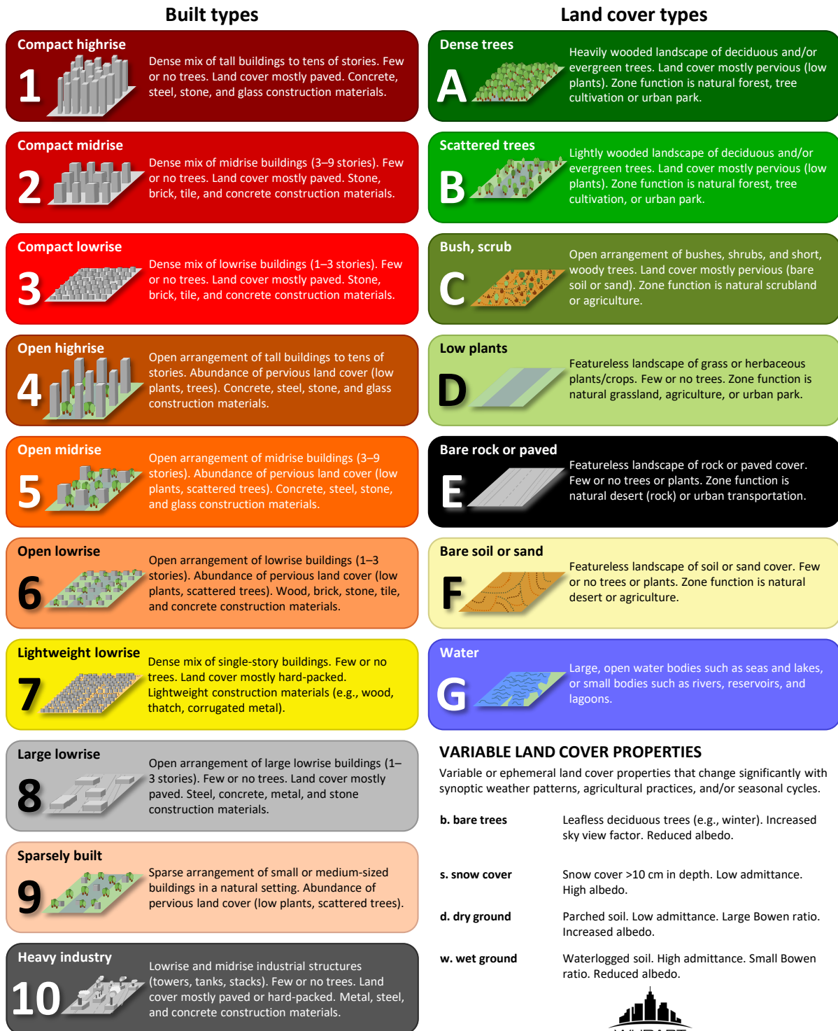
Figure 1. Definitions of built (1-10) and land cover types (A-G) for the Local Climate Zone scheme (Stewart and Oke, 2012; Demuzere et al., 2020a).
