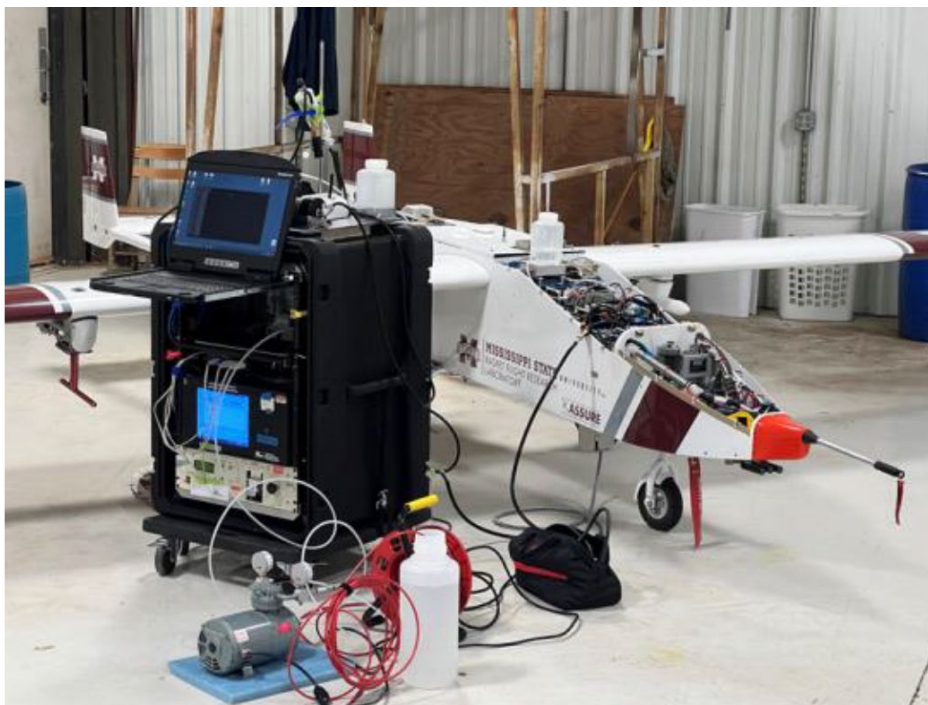
Figure 3. the AAF UAS payload sensors installed on the MSU TigerShark were compared with the PNNL aerosol ground mobile station (AGMS) before each flight.
