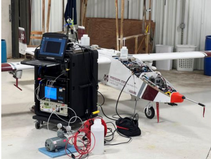
Figure 3. the AAF UAS payload sensors installed on the MSU TigerShark were compared with the PNNL aerosol ground mobile station (AGMS) before each flight.
