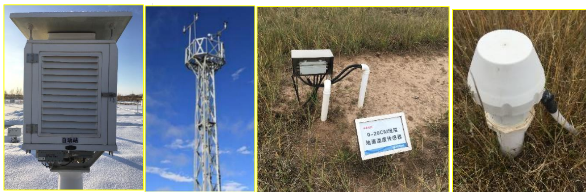
252 Figure 6. Instruments for observation of (a) air temperature and wetness, (b) wind speed, (c) soil temperature 253 and (d) soil moisture.
