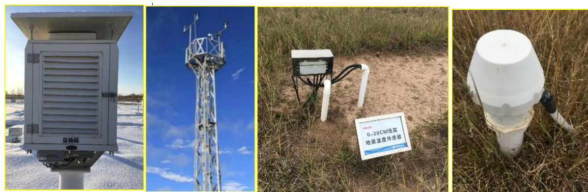
Figure 6. Instruments for observation of (a) air temperature and wetness, (b) wind speed, (c) soil temperature and (d) soil moisture.
