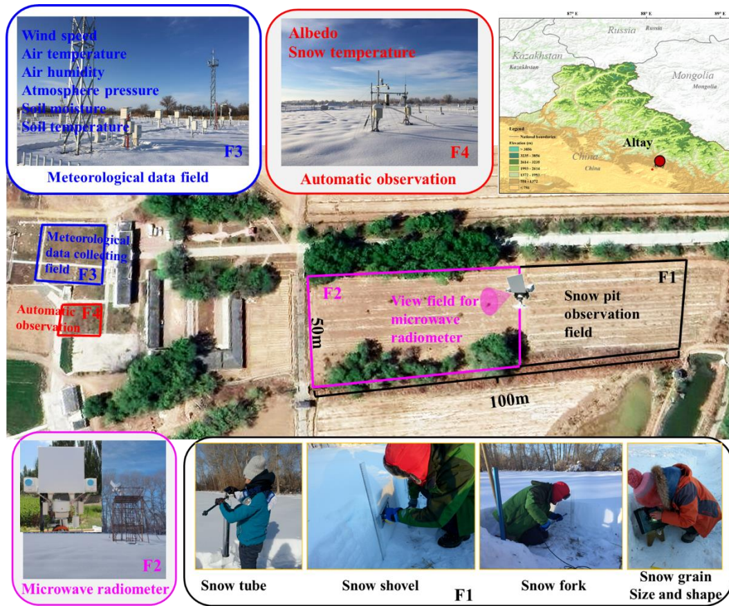
121 Figure 1. Location of the Altay National Reference Meteorological station (ANRMS) in Asia, along with the 122 four test sites in the ANRMS. The black-rectangle field F1 (approximately 40 m × 50 m) was for snow layering, 123 layer thickness, snow density, snow grain size and shape of each layer. The pink-rectangle F2 (approximately 124 60 m × 50 m) was for microwave radiometers observations. The blue-rectangle field F3 was for meteorological 125 and soil data collection operated by the ANRMS. The red-rectangle F4 was for the automatically observation 126 of the snow temperature, and 4-component radiation, designed by Northwest Institute of Eco-Environment 127 and Resources, Chinese Academy of Science (NIEER).
