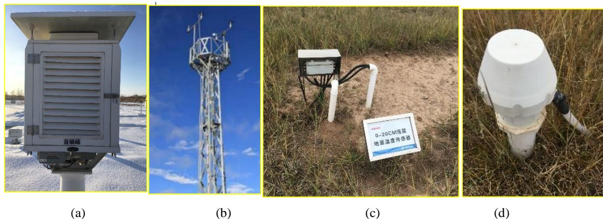
Figure 6: Instruments for observation of (a) air temperature and wetness (a), (b) wind speed (b), (c) soil temperature (c) and (d) soil moisture (d).
