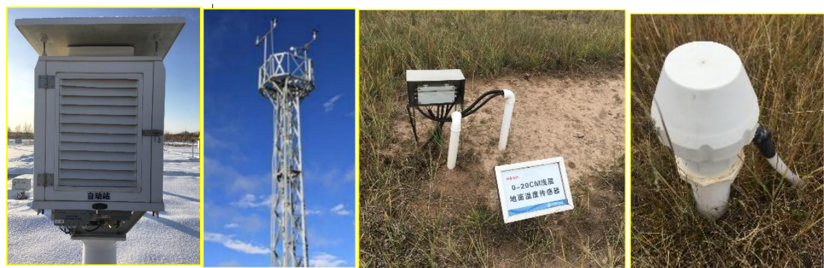
288 Figure 6: Instruments for observation of air temperature and wetness (a), wind speed (b), soil temperature 289 (c) and soil moisture (d).
