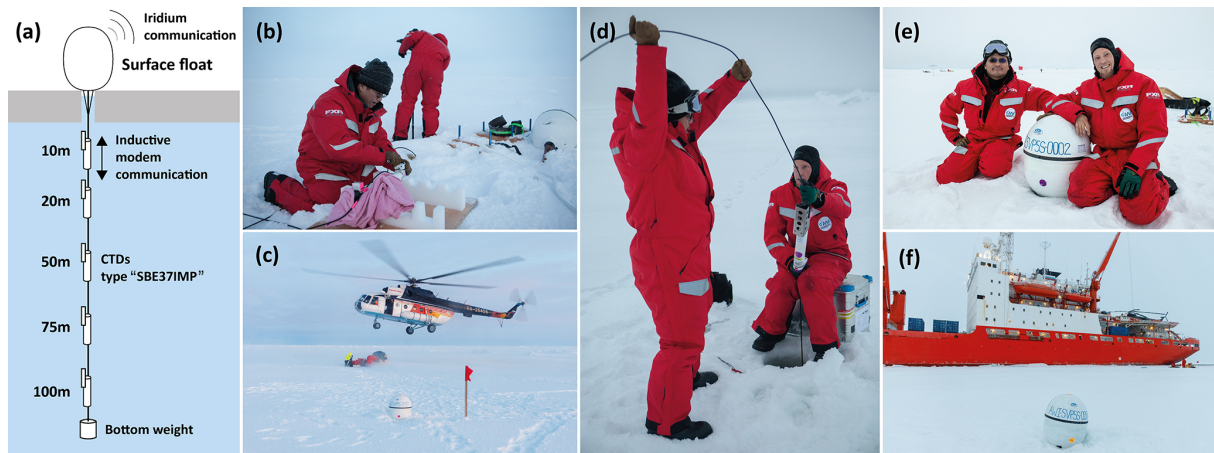
Figure 1. Salinity ice-tethered buoy schematic (a) and deployment photos (b–f).
