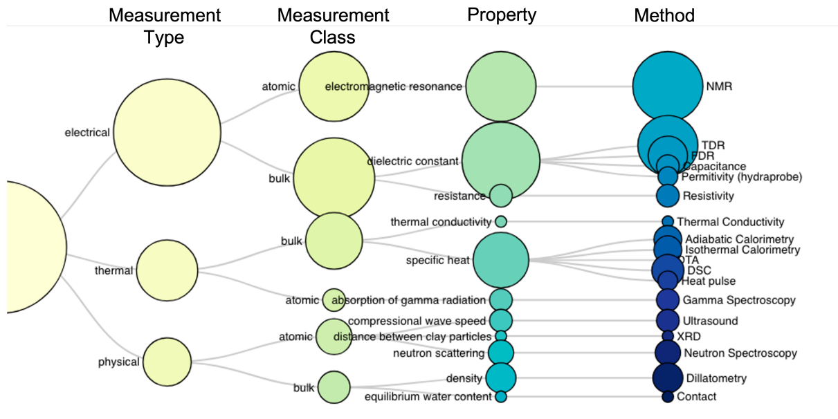
Figure 2. Organization of measurement methods according to measurement principle. Size of nodes represents the relative number of SFCCs collected using each method.
