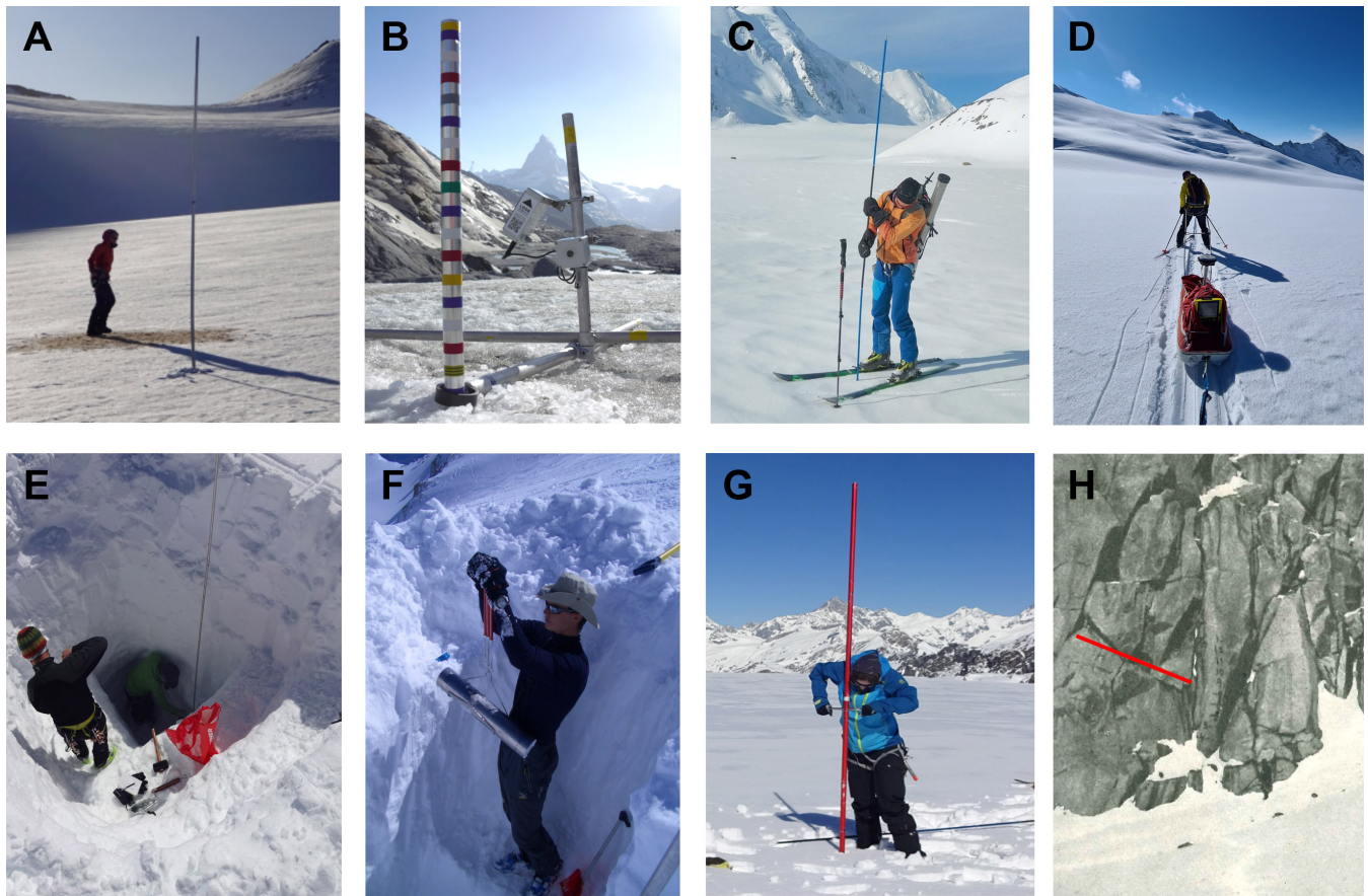
Figure 3. Illustration of different methods of point mass balance data acquisition: (A) Mass balance stake and marked horizon (accumulation area), (B) ablation stake with markers and automated camera-based readings, (C) snow probing, (D) ground-penetrating radar for measuring snow layer thickness, (E) snow pit excavation, (F) snow density measurement in a snow pit, (G) coring for snow density measurement, (H) historic method of nivometers (markers painted on vertical, ice-marginal rocks). Photos: M. Huss (A,E-G), C. Ogier (B-D), P.-L. Mercanton (H).
