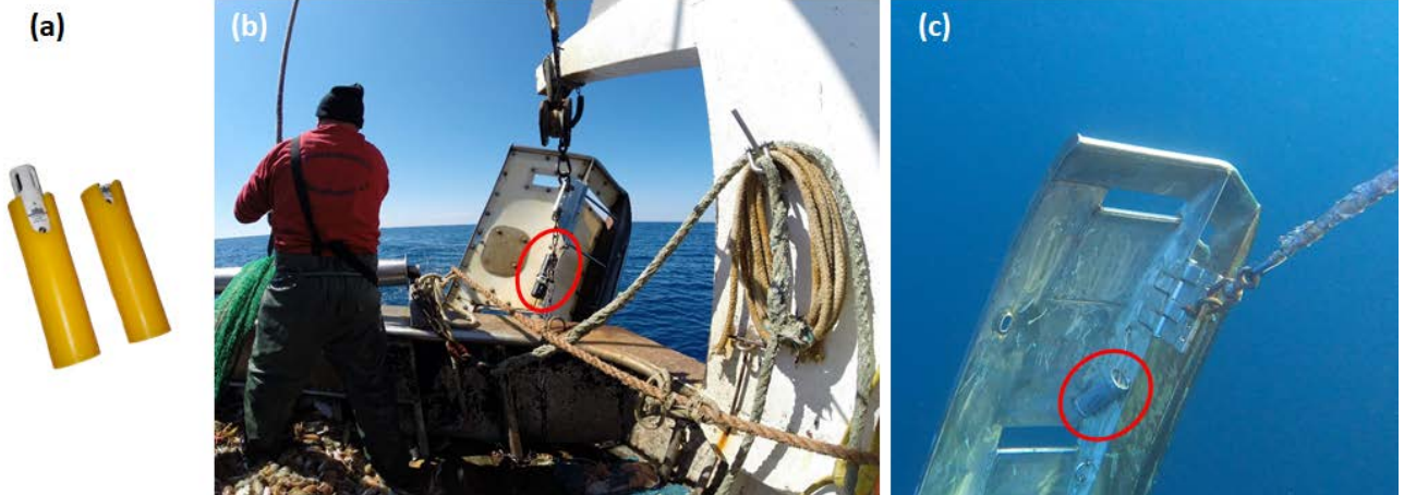
Figure 3. NKE SP2T and STPS sensors inserted into yellow rubber protections supplied by the company (a) installed on the otter door of a commercial bottom trawler (b); otter door and sensor during the fishing operation (c).
