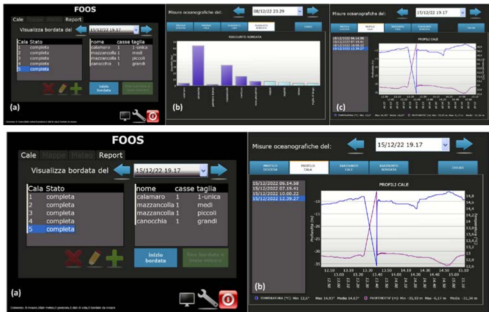
175 Figure 4. AdriFOOS GUI used onboard by fisherman: screenshot examples from the catch module (a) allowing to enter the start/end of the trip (in Italian Inizio/Fine bordata ) and caught species quantity ( casse ) and size ( taglia ) by haul (Cala)-(a, b) and the oceanographic real time data visualization module (b) showing fished depth (purple line) and relative temperature (blue line) by haul.
