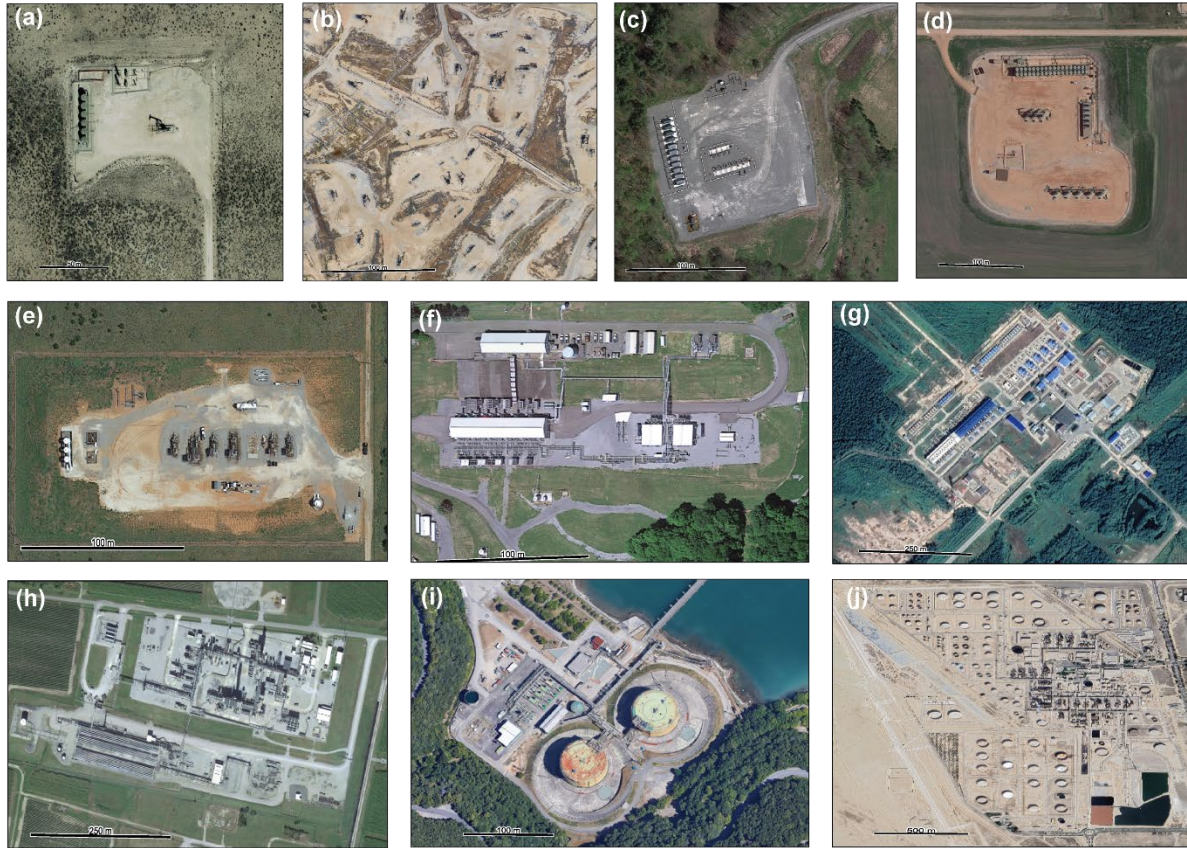
Figure 1. Examples of major oil and gas facility types as seen in high-resolution satellite imagery (Google basemap imagery, © Google Earth). (a). An oil well pad with one pump jack and storage tanks in the Permian Basin, U.S. (b). A cluster of oil pumpjacks in Kern River Oil Field in California, U.S. (c). A dry natural gas production well pad, with 11 horizontally-drilled wells, in the Marcellus Shale play (northeastern Pennsylvania, U.S.). (d). A mixed oil and gas production well pad in the Bakken Shale play (North Dakota, U.S.), with eight horizontally-drilled wells. (e). A natural gas gathering compressor station in the Anadarko Basin (Oklahoma, U.S.). (f). A natural gas transmission compressor station in Pennsylvania (U.S.). (g). A natural gas transmission compressor station in West Siberian region (Russia). (h). A natural gas processing plant in Louisiana (U.S.). (i). An LNG regasification facility in La Spezia, Italy. (j). A crude oil refinery in Mesaieed, Qatar.
