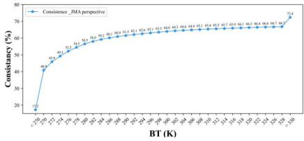
Figure 10: The variation of consistence between JMA-Himawari-8 and NSMC-Himawari-8 fire product under different brightness temperature.
