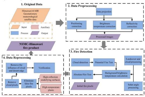
Figure 2: General flowchart for generating NSMC-Himawari fire products.
