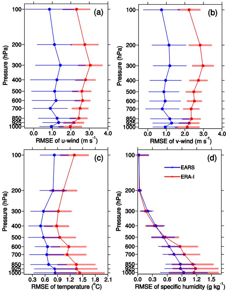
**Fig. 13** Comparison of averaged RMSEs of EARS (blue) and ERA-Interim (red) at different levels for (a) u-wind ( $U$ ;  $\text{m s}^{-1}$ ), (b) v-wind ( $V$ ;  $\text{m s}^{-1}$ ), (c) temperature ( $T$ ;  $^{\circ}\text{C}$ ), and (d) specific humidity ( $Q$ ;  $\text{g kg}^{-1}$ ). The standard deviation of RMSE at each level is marked by a horizontal line.
