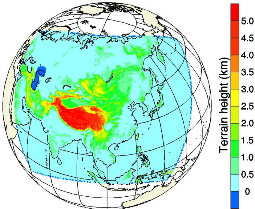
825 **Fig. 1** The East Asia Reanalysis System (EARS) domain in the WRF model, and its 12-km topography. The shading indicates the height of the terrain in the model.
