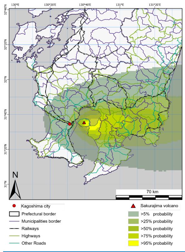
Figure 7. The probability distribution of ash dispersal with the threshold for road closure risk ( \geq 3 cm). Black and white stripes mark railways on the map, and highways and other roads are in coloured lines. The colour gradient shows the difference in the probability of ash deposits exceeding the threshold. Human geography base is used as the basemap for this figure (ESRI, 2022).
