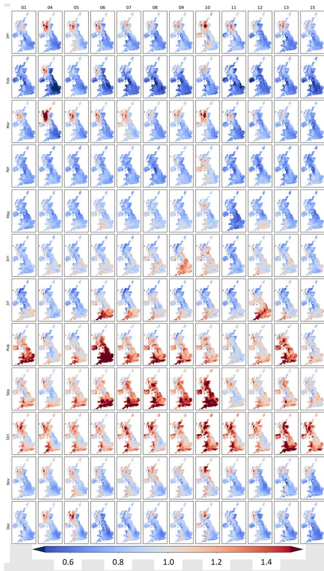
Figure 2: Bias-correction grids applied to correct monthly precipitation. Values are correction factors used to modify precipitation, with a value of 0.5 halving precipitation, 1 meaning no change to precipitation and 2 doubling precipitation etc. Columns show results from each RCM PPE member, rows show results for each month. Note the column numbers reflect the RCM PPE number descriptor for each RCM run – (see Sect. 3) and are not sequential (i.e. there is no 2, 3, or 14 and so the numbers run to 15, but there are actually only 12 columns)
