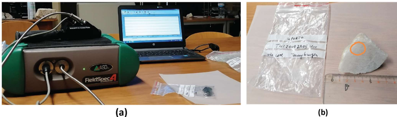
Figure 2: (a) FieldSpec 4 (ASD, Inc.) standard resolution spectroradiometer. (b) Example of an annotated photograph of the measurement spot in a sample from Tysfjord. A similar photograph accompanies each analysed spot in the spectral library.
