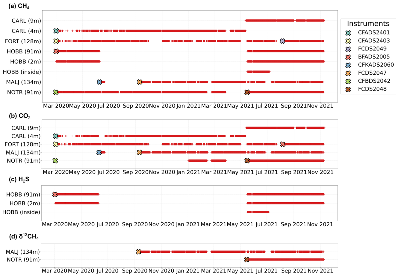
Figure 4: Data availability and instruments used at each site. Inlet level (meters above ground level) is indicated besides the site name. (a) Methane (CH 4 ) data availability at all sites. (b) Carbon dioxide (CO 2 ) data availability. (c) Hydrogen sulfide (H 2 S) data availability. (d) Methane isotope (δ 13 CH 4 ) data availability. At the sites with more than one level of measurement (e.g., HOBB and CARL), all the levels operate using the same instrument at that site. Instruments replacements were made due to instrument failures at FORT, MALJ and NOTR.
