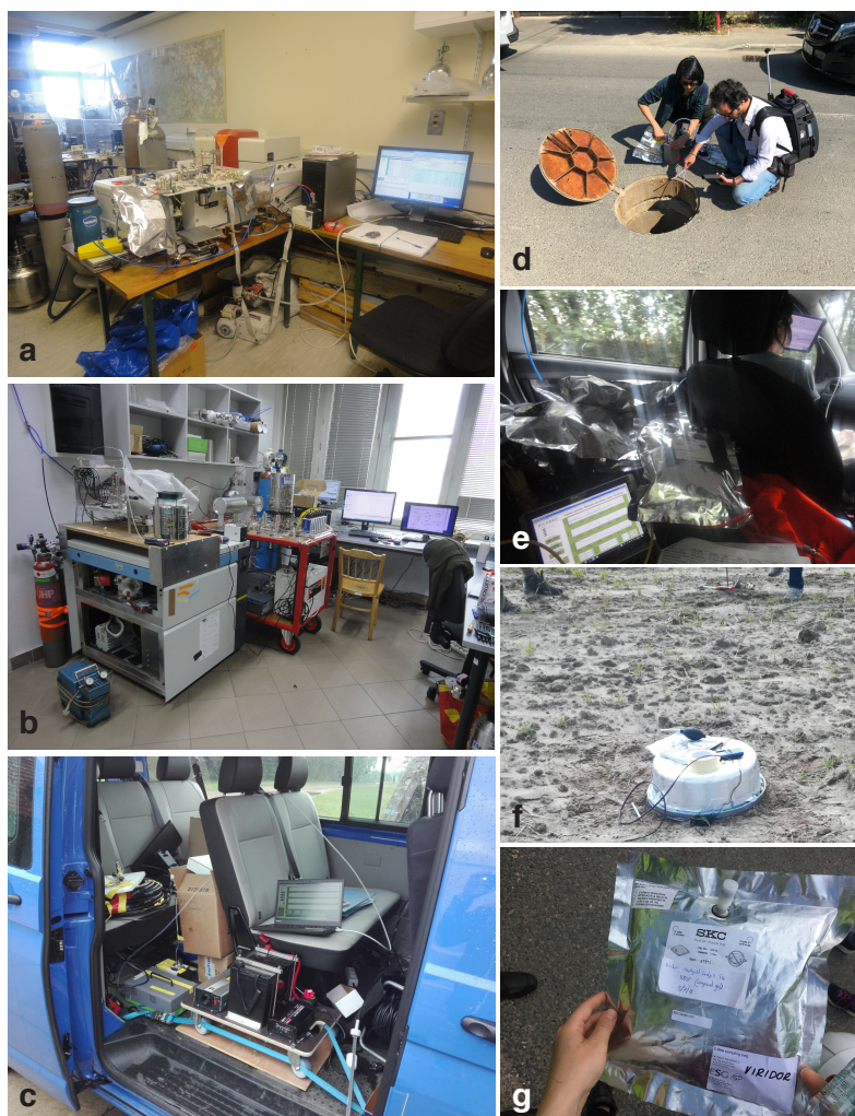
Figure A1. Photos of the laboratory setup used for isotopic measurements during the MEMO 2 project and of the sample collection during field surveys. (a) IRMS system setup used at GGRL RHUL, for \delta^{13}\text{C}_{\text{CH}_4} measurements. (b) IRMS system setup used by the UU team, here deployed at Krakow, for \delta^{13}\text{C}_{\text{CH}_4} and \delta^2\text{H}_{\text{CH}_4} measurements. (c) Mobile measurement setup used by the Heidelberg University (UHEL) team, using cavity ring-down spectrometry (CRDS) isotope analyser and an air-core, as described in Hoheisel et al. (2019). Photo: Piotr Korbeń (d) Sample collection directly from an emission source on foot: a manhole in the city of Bucharest, Romania. \text{CH}_4 mole fractions were measured using a portable CRDS analyser. Photo: Octavian (e) Mobile measurements and sampling on-board of a car. Air was pumped from the top of the car and continuously measured with a CRDS analyser, and bag samples were taken when \text{CH}_4 enhancement were detected by the instrument. (f) Soil chamber placed on a coal waste disposal area in Poland. Samples were collected from the chamber several hours after it was placed. \text{CH}_4 mole fractions in the chamber were measured using a portable integrated cavity output spectroscopy (ICOS) instrument. Photo: Mila Stanisavljević (g) Full sample bag before analysis, collected on a landfill in Devon, UK.
