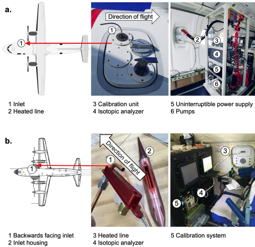
Figure 5: Water vapor isotopic sampling installations on the a) ATR and b) P-3 aircraft. (ATR schematic downloaded from <https://t3projects.mpimet.mpg.de/coordination/platform-schematics>. P3 schematic provided by NOAA.)
