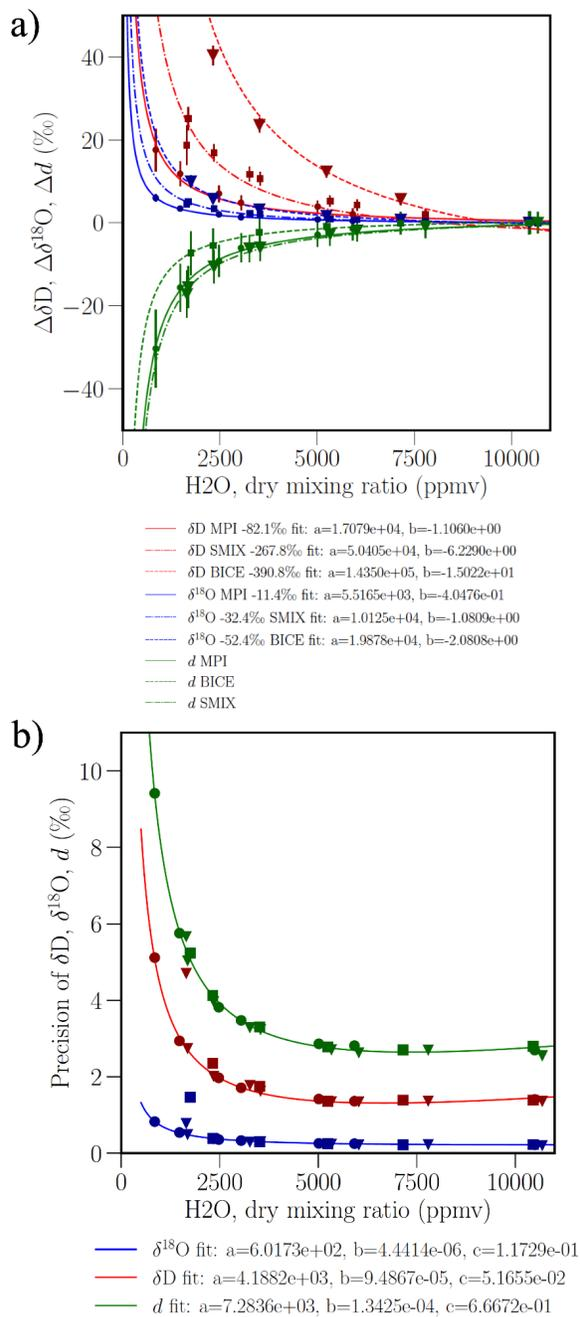
1455 **Figure 7: Bias corrections and uncertainties associated with the ATR water vapor isotopic measurements: a) symbols illustrate the humidity dependence of the isotopic measurements for three distinct liquid standards (MPI, SMIX, BICE) while lines show the correction functions used to remove the detected biases in  $\delta^{18}O$  (blue) and  $\delta D$  (red); b) precision of the isotopic measurements as a function of the measured water vapor concentration.**
