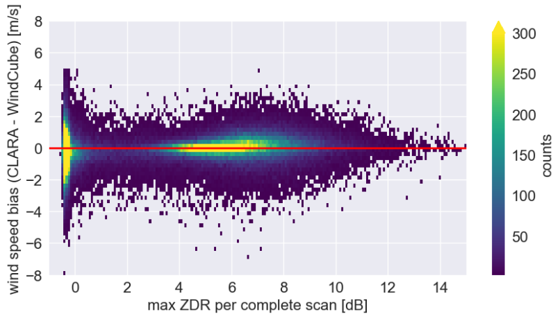
Figure 7. Two-dimensional histograms of the difference between WindCube's and CLARA's wind speed from the lowest 2 km as a function of the maximum ZDR. Note that only data with I_{inv} smaller than 50% is used.
